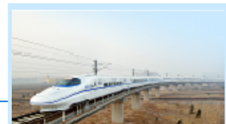
Harmony extended trains (16-units) with speed of 200-250 km/h, which is China's first multiple unit developed with independent intellectual property
