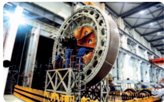
• 6MW direct-drive permanent magnet synchronous generator stator manufacturing lens
